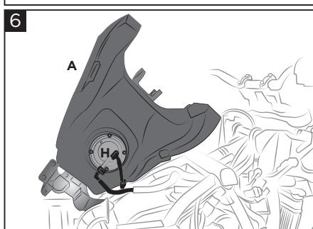
**Connect the connectors to the pump (H) first to mount the tank (A).**
