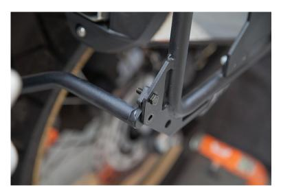
13. After lining up the mounting holes, go ahead and insert the 6x20mm hex head bolts and secure them using the provided washers and locking nuts.
