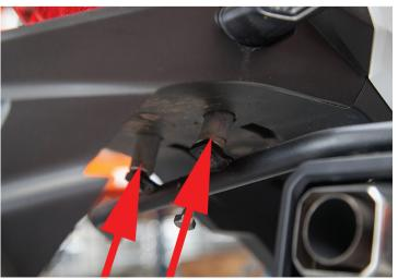
3. Insert the washers and thread both M8 locking nuts on the top side of the fender where the passenger seat's been removed. Leave them loose.
