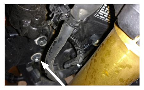
Remove the lower of two M8 hex cap screw (12mm socket) that attaches the front fairing bracket to the bike frame at the head stock. You will not need this later.
