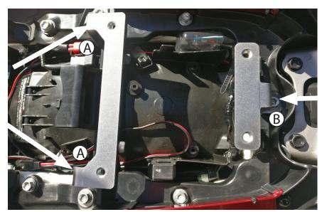
(A)Install front bracket as shown with OEM M6 hex screws from step 1.
