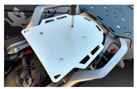
Use 5mm allen tool with M8 x 16mm flat head screws to install rack platform. Attach front seat.
