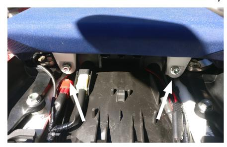
Remove front seat. Use 10mm socket to remove M6 hex screws and remove the pillion seat. Save these screws for later.
