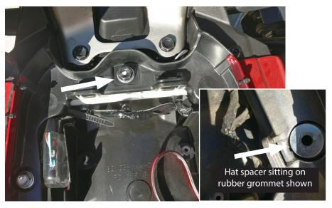
Use 12mm socket to remove the one M8 bolt as shown. The OEM hat spacer and rubber grommet that are below the washers stay and the bracket will mount on top.
