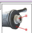
OEM bar-end weight removed
