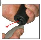
Neatly cut Diameter 25 to 26mm hole in end grip
