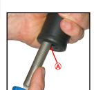
File away any burrs from inside the handlebar end
