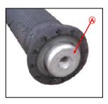
OEM bar-end weight removed
