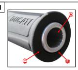
OEM bar-end weight removed
