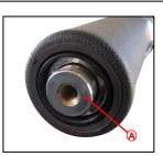
OEM bar-end weight removed
