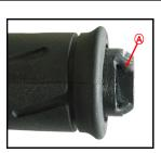
OEM bar-end weight removed with tapered stub
