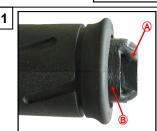
Tapered 18.7mm stub end with OEM bar-end weight removed
