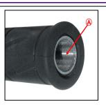
OEM bar-end weight removed (Hex plug also removed)
