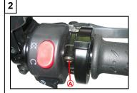
Throttle assembly clamp screws
