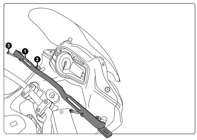
**Step One:** Using the supplied hardware mount the light bracket to the motorcycle as illustrated above.
