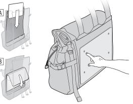
Use a ball point pen to mark hole locations where the mounting hardware passes through the Pannier. Repeat on second Pannier.
