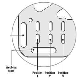
Use one of the three slot positions to locate mount hooks where they clear obstructions and hot exhaust. Adjust hooks vertically in slots for a tight fit when the quick-connect clasp is attached to the rack.
