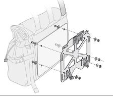
INSTALL ONTO LUGGAGE RACK Once GL Pannier Mounts are installed on RTW Panniers, hold by the handle and drop hooks onto luggage rack, pulling quick-connect clasp open and allowing it to click into place. Lock Panniers to luggage rack for maximium security and to prevent accidental disconnection of Pannier Mount.
