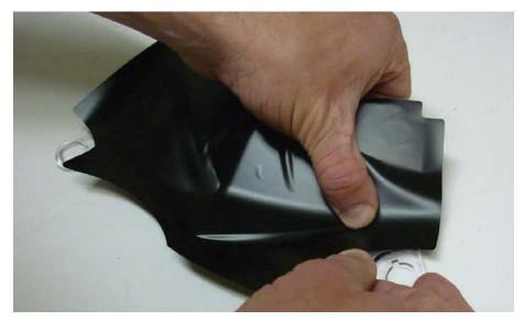
Continue to work from the center outward with your thumb or fingers, pressing out bubbles to the edge while lifting with your other hand. It may be lifted and repositioned as necessary to get it to lay smoothly. Large bubbles can be carefully pricked with a sharp exacto knife and pressed flat.
