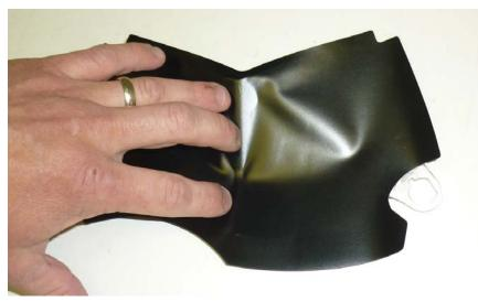
(2) Attach sticker starting with the center ridge. The sticker is larger than the deflector and there should be some overhang on the edges. Press into the crosswise bend. Use your finger to press into place, pulling on the sticker edge with your other hand as necessary.
