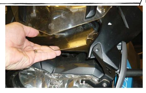
Remove clear wind deflector by unscrewing the same two T25 torx that hold the headlight guard brackets on. Clean the wind deflector with warm soapy water. Dry. Keep your hands clean.
