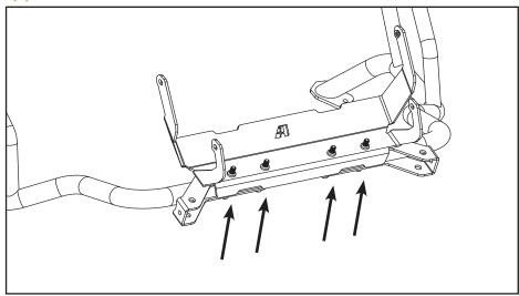
Place the AltRider light mount brackets around the tube, and sandwich them to the under-nose bracket. Install the M6 x 50mm socket cap screws with washers. Torque to 8.7 Nm.
