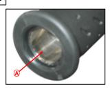
OEM bar-end weight removed
