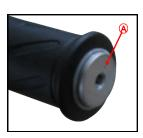
OEM Bar-end weight removed
