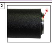
Re-pin Throttle assembly so that handle bar protrudes by 2,5mm
