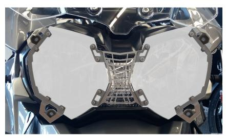
Install headlight guard. !TIP A dab of water on each ball stud will help it fit in place easier with less wear on the rubber grommets.
