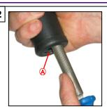
File hole in the throttle sleeve to the same inside diameter as handlebar tube
