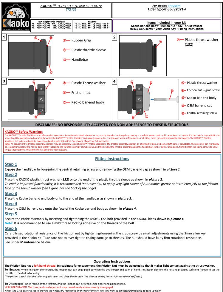
Maintenance: Remove kit annually. Unscrew Friction Nut and brush clean threads with a mild soap. Apply petroleum jelly to threads and assemble. Adjust grub screw to desired operating resistance. (O-Ring cushion: 19.6mm I.D. x 2.4mm section — if replacement is required)
