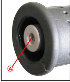
**A** — OEM bar-end weight removed
