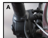
Step A : Loosen throttle assembly clamp screws
