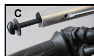
Step C : Fit an M6 bolt into newly exposed threaded insert. Insert is now exposed after trimming throttle sleeve and rubber grip, and then removing the throttle assembly.
