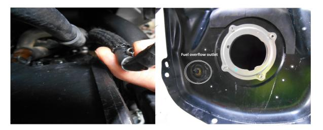
6. Install the Safari tank onto the motorcycle by angling the tank from the righthand side of the motorcycle and raising the back of the tank to allow it to fit pass the posts on the plastic fairing tower.
