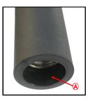
OEM Bar-end weight removed
