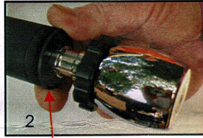
Thrust Washer—recess Facing Throttle Sleeve
